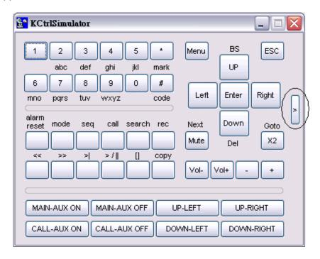
Note that most of the Keys correspond to the keypads on the front panel. If you connect the PC through RS-232 and use an RS-232/RS-485 converter to connect to multiple DVR/NVRs, you would be able to control multiple DVR/NVRs via the simulation software. Refer to <a href="Section 3.2 Optional Connections">Section 3.2 Optional Connections</a> to connect/cascade the DVR/NVRs to the PC.
