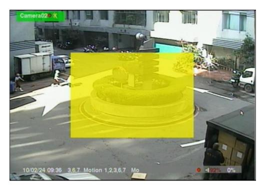
The system supports X2/X4 Digital Zoom function. To use this function, press X2 Key (Mouse: in full screen display to enter Digital Zoom mode. There will be a zoom window shown in the video window as shown. The zoom window (a) will always be shown at zoom factor X1, (b) can be shown or hidden at zoom factor X2, and (c) will never be shown at zoom factor X4. The operations in Digital Zoom mode are as below:
