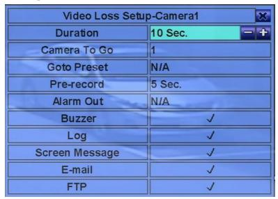
In Camera Setup, press **ENTER** to call up Video Loss Setup of the selected camera as shown when the highlighted option is **Video Loss Settings..** of the camera to setup. The Video Loss Setup allows the administrator to define how the system responds to the detected video loss for the camera.
