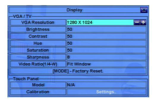
In Menu display, press  $\blacktriangle \lor \blacktriangleleft \blacktriangleright$  to change the highlighted option to Display, and then press ENTER to call up Display dialog as shown. There are several items which can be adjusted, including Resolution, Brightness, Contrast, Hue, etc. Besides, Touch panel models are also supported.
