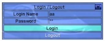
In Login/Logout display, follow the Text Input method described in <u>Section 4.1</u> to enter the **Login** name and **Password**, press ▲ ▼ to highlight and select **Login** option, and then press **ENTER** to login the system. If the user wants to logout the system, just press ▲ ▼ to highlight and select **Logout** option, and then press **ENTER**. Press **ESC** to exit without making changes.
