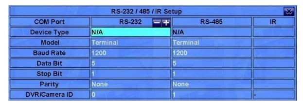
The RS-232 / 485 / IR Setup allows the administrator to setup RS-232 / 485 / IR control port and NVR ID for IR remote. Refer to the manuals for the connected devices - PTZ cameras or keyboard Controls – to set the items in RS-232/485 Setup.
