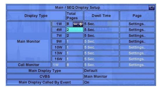
The Main/SEQ Display Setup allows the administrator to define the display pages in SEQ Display for main monitor and call monitor. Note that Call Monitor supports 1/4 split window display.
