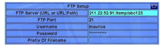
The FTP Setup allows the administrator to set FTP related parameters. When an event occurs and FTP is enabled for the action, the recorded video/audio for that event will be sent to the FTP server based on the parameters set here.
